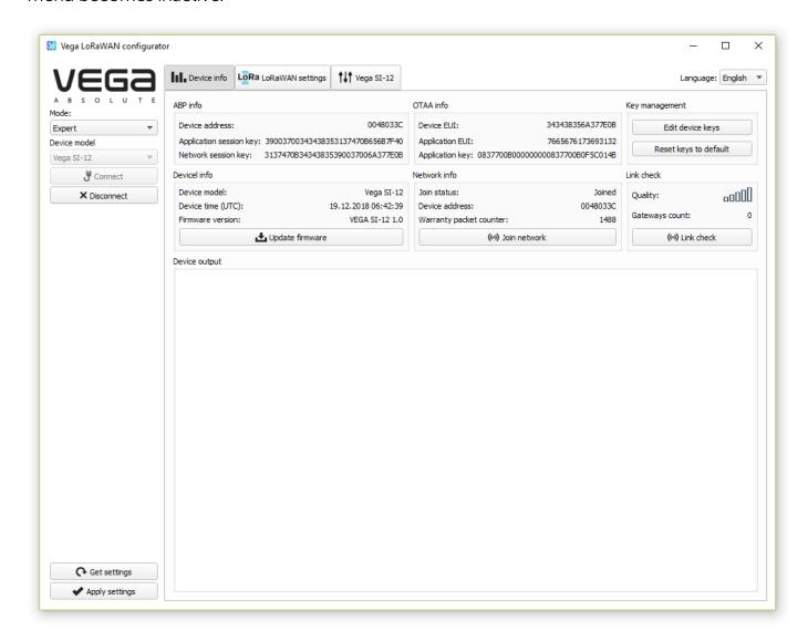
To read the settings from the device, you need to click the "Get settings" button, until this point the application will display the default settings or from the last connected device.
