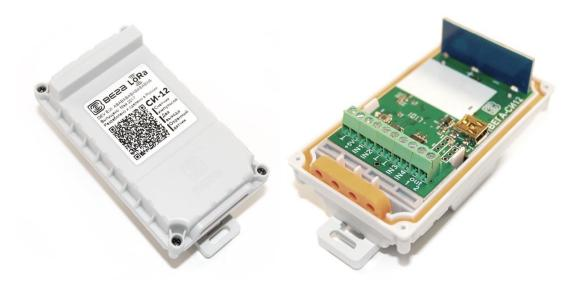
The counter is powered by a 3400 mAh built-in battery with service life up to 10 years, provided data transmitted once a day. The counter can be powered by the 5V external power supply.
