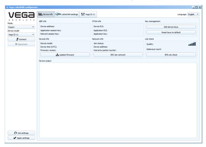
The menu on the left allows you to switch between the "Simple" and "Expert" modes, select the device model, connect to the device or disconnect from it, get and apply settings.
