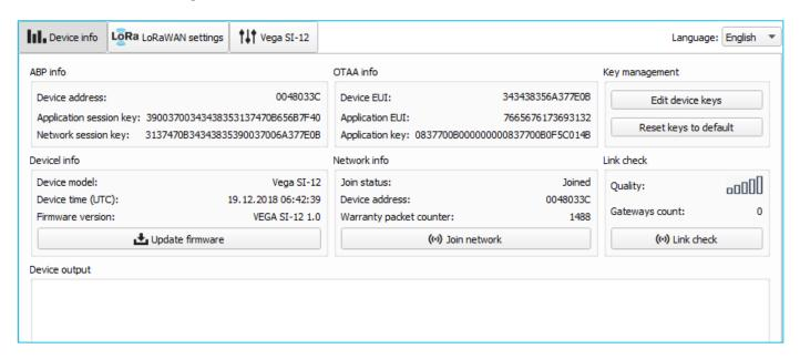
**ABP info** - displays the data necessary to register the device in the LoRaWAN network with ABP method (Activation By Personalization).
