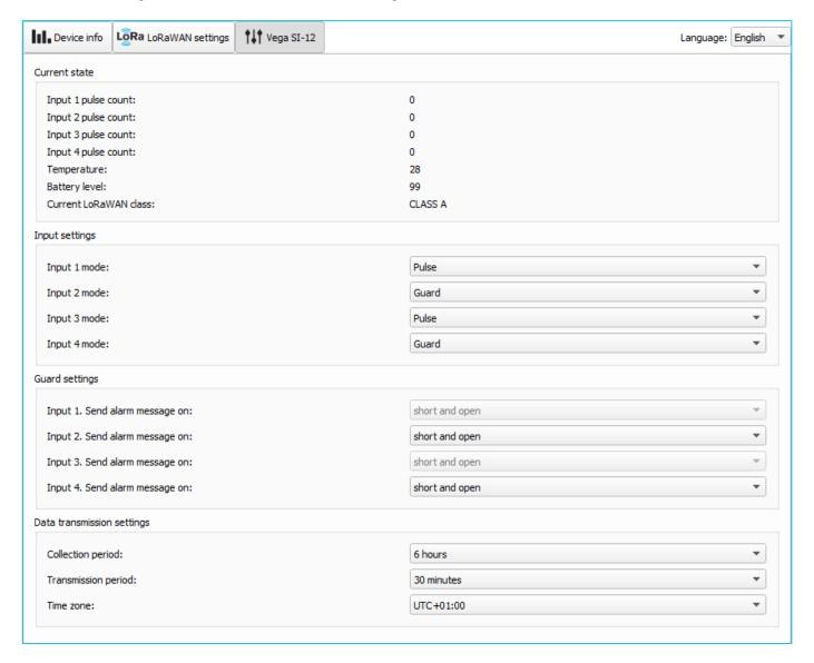
Current state – displays the current parameters of the device - the number of counted pulses at the inputs, the temperature, the battery level and the current LoRaWAN class.
