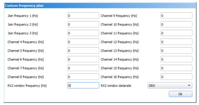
This frequency plan allows you to set up to 16 channels, as well as the frequency and speed of the second receiving window.
