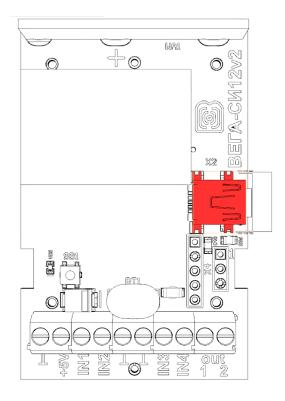
Before connecting the device to the computer for the first time, you must install the driver for the COM port **stsw-stm32102**, which can be downloaded from iotvega.com. After running the executable file **VCP\_V1.4.0\_Setup.exe**, the installer window will appear:
