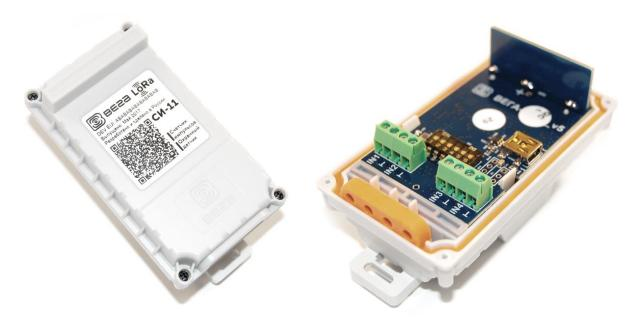
The counter is powered by a 3400 mAh built-in battery with service life up to 10 years, provided data transmitted once a day.
