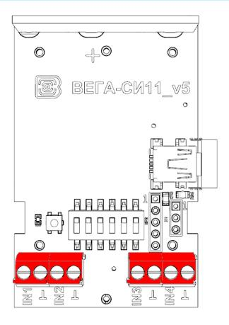
The pulse counter has 4 pairs of contacts and is able to connect circuits with the following types of NO contacts:
